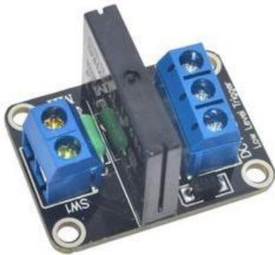
Gambar 5.1 *Solid State Relay (SSR)*
